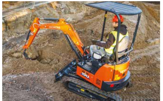
Three-post canopy design enhances visibility.
