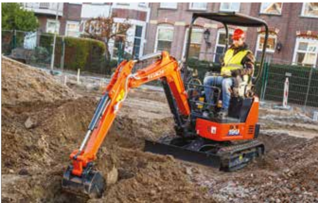
Expandable crawler tracks enhance versatility and stability.
