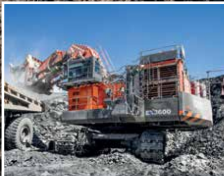
EX ultra-large excavators
