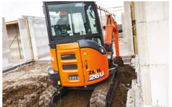
Short-tail swing radius is ideal for working in narrow spaces.
