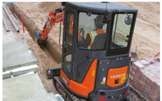
The short-tail swing radius makes the ZX33U-6 ideal for working in tight spaces.
