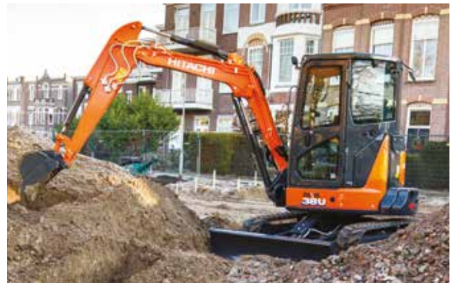
The short-tail swing radius makes the ZX38U-6 ideal for working in tight spaces.
