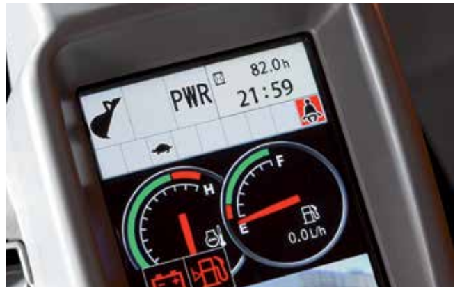
Large color multifunctional LCD monitor shows data at a glance.
