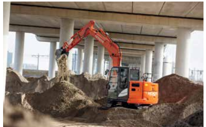
The short-tail swing radius makes the ZX85USB-6 for working in tight spaces.
