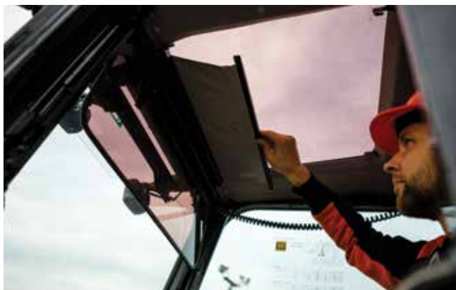
The sun visor reduces glare from the sun and enhances visibility.
