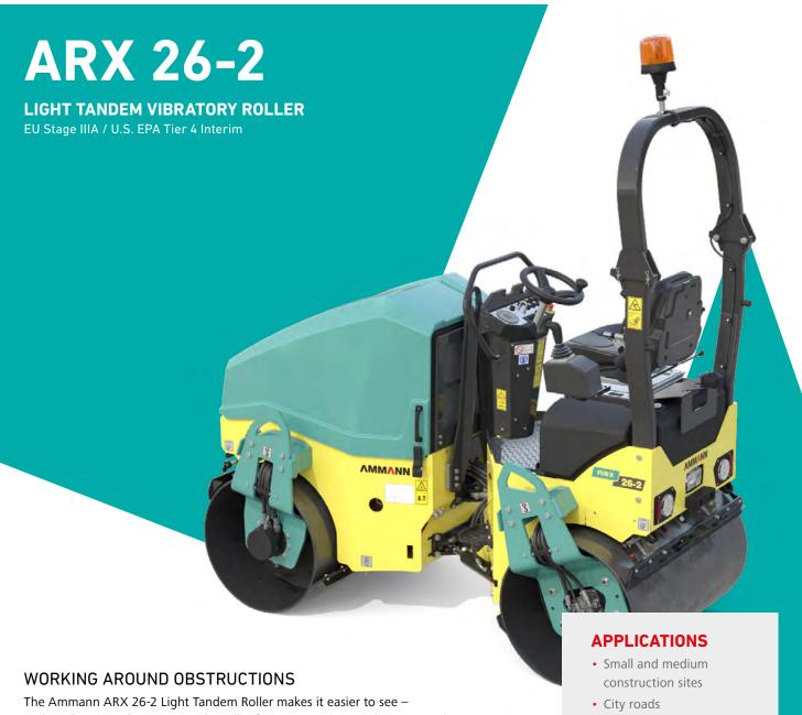
The Ammann ARX 26-2 Light Tandem Roller makes it easier to see — and work — near obstructions. The roller features a new articulation joint that enables quick drum adjustment from in-line to offset configurations, helpful when working close to obstructions. Operators need watch only one drum, knowing the second will be a safe distance from the obstacle. The in-line drum setting is available when it's time for productivity in open spaces.
