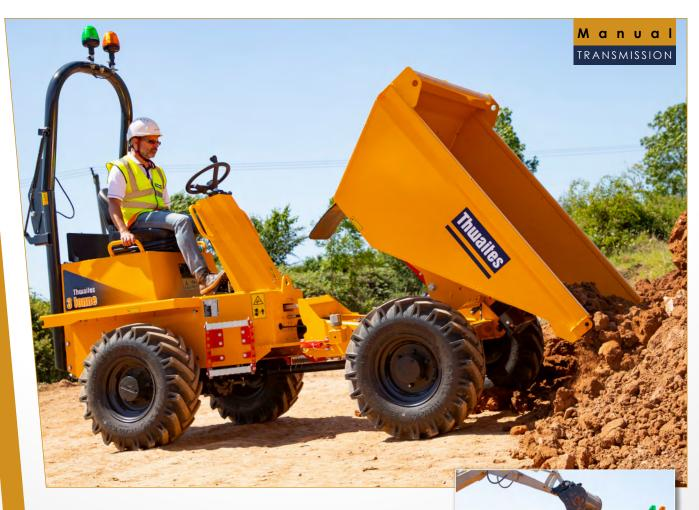
The Thwaites 3 Tonne Front Tip, Stage V dumper is manufactured with contractors and hirers in mind – ensuring operator safety, reducing risk on site and improving performance. Powered by an 18.4 kW Yanmar engine, delivering 107 Nm max torque for optimum traction and control. This machine is driven by a Manual transmission.
